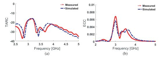
Figure 11. Calculated (a) TARC, (b) ECC results of the adjacent elements.
