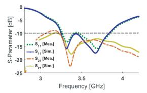
Figure 9. S-parameters of the adjacent PIFAs.
