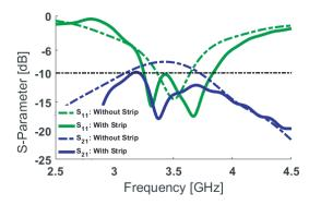
Figure 2.  $S_{11}/S_{21}$  of adjacent elements with/without the arrow-strip.
