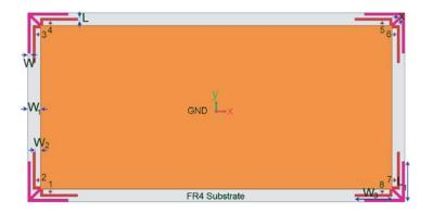
Figure 1. Configuration of the smartphone antenna array.
