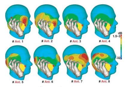
Figure 14. Radiation patterns at 3.5 GHz in Talk-Mode.
