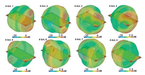
Figure 5. 3D radiation patterns of the PIFAs at 3.5 GHz.
