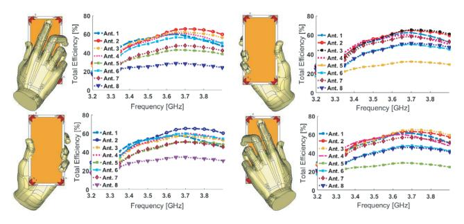
Figure 12. Placement and efficiencies of the PIFA array at different user-hand scenarios.
