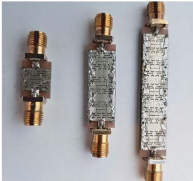
Figure 15. A photograph of the fabricated SIW-metamaterial filters.
