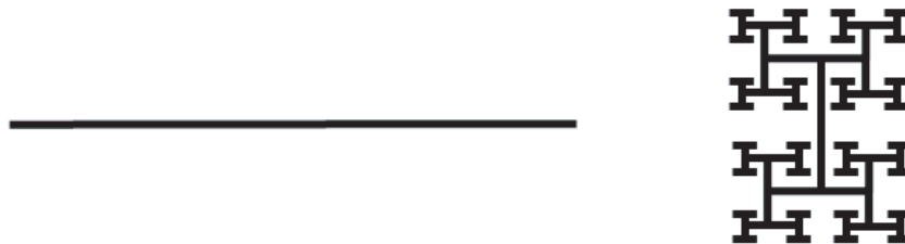
Figure 1. A comparison between the conventional straight-line (e.g., transmission-line) and its length-equivalent fractal curve.
