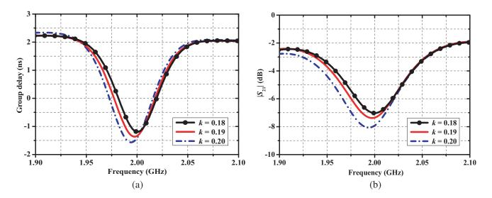
**Figure 4.** Effect of k on the performances of the proposed NGD bandpass filter. (a) Group delay. (b)  $|S_{21}|$ .
