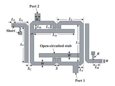
Figure 1. Configuration of the proposed NGD bandpass filter.
