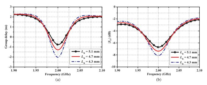
**Figure 3.** Effect of  $L_R$  on the performances of the proposed NGD bandpass filter. (a) Group delay. (b)  $|S_{21}|$ .
