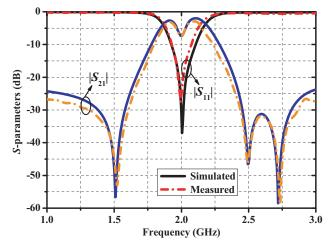
Figure 9. Simulated and measured S-parameters of the proposed NGD bandpass filter.
