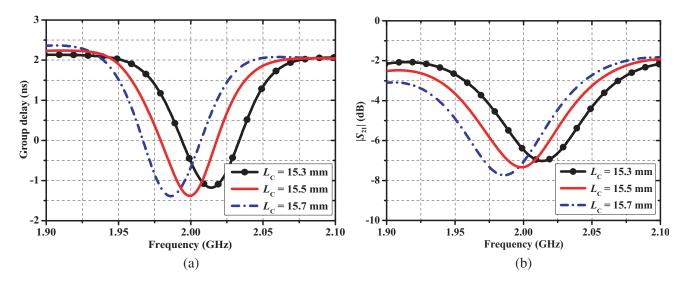
**Figure 5.** Effect of  $L_C$  on the performances of the proposed NGD bandpass filter. (a) Group delay. (b)  $|S_{21}|$ .
