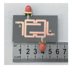
Figure 7. Photograph of the proposed NGD bandpass filter.
