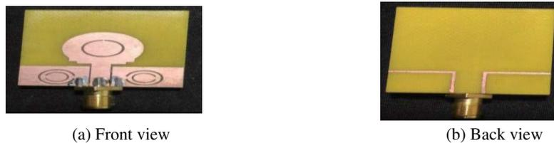
Figure 4. Fabricated model of a semi-circular UWB antenna.
