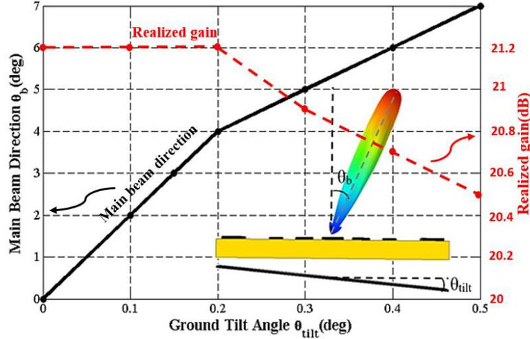
**Figure 10.** The linearity of beam scanning as a function of ground tilting angle.
