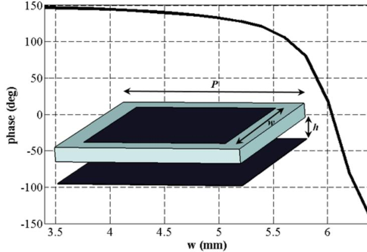
**Figure 4.** Unit cell and phase diagram as a function of patch width at 9.5 GHz.
