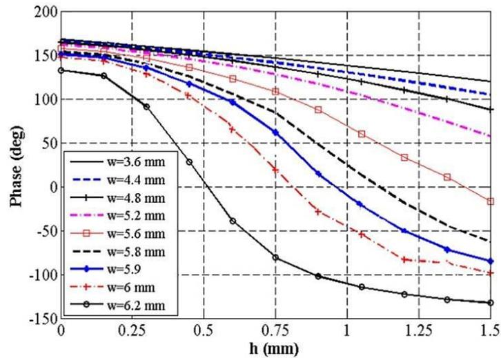
Figure 5. Phase- $h$  curves for different patch widths.
