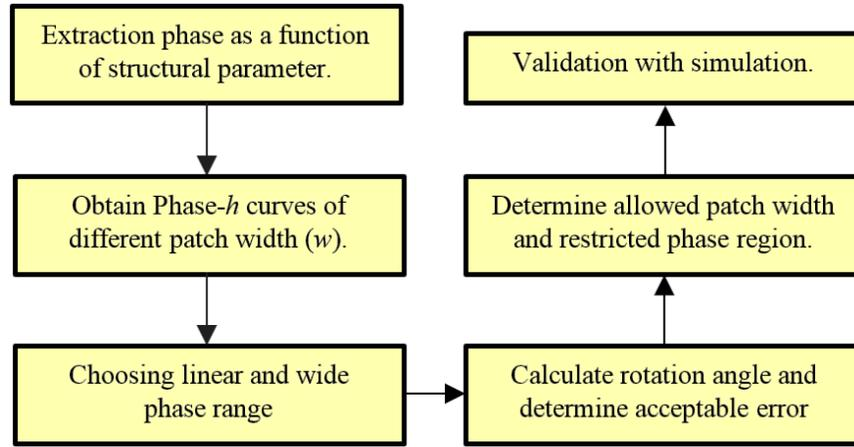
Figure 2. Design procedure of the steerable non-uniform reflectarray.
