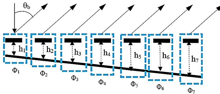
**Figure 1.** Schematic reflectarray and their element phase.
