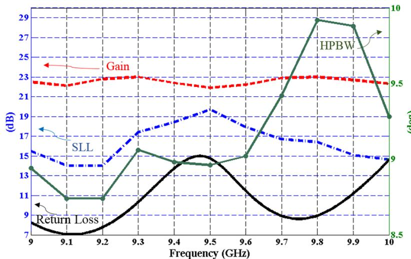
**Figure 9.** Antenna gain, HPBW and SLL as a function of frequency.
