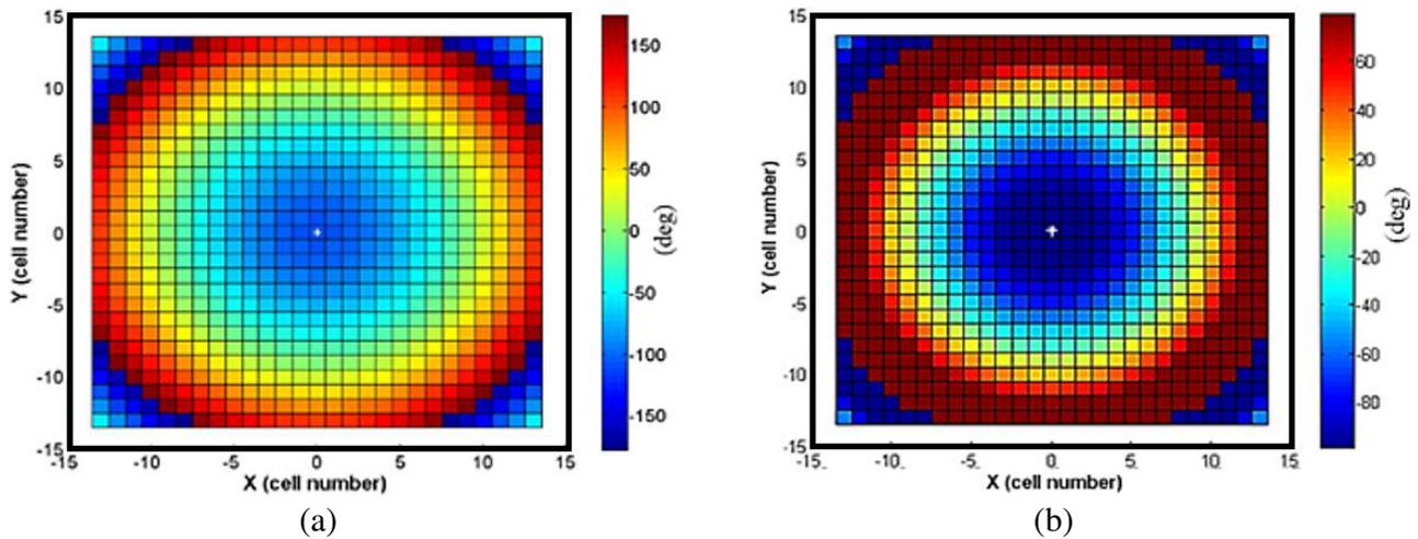
Figure 6. Phase distribution on the antenna aperture. (a) The required phase distribution on reflectarray antenna surface. (b) The required phase restricted between  $-100^\circ$  to  $80^\circ$ .
