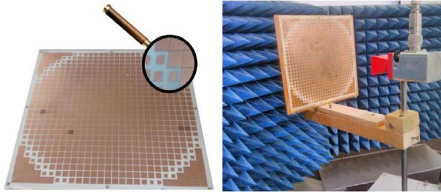
**Figure 7.** Prototype of fabricated reflectarray and test setup.
