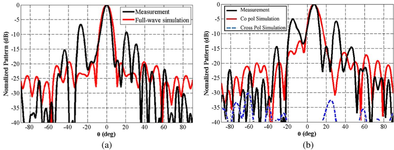
**Figure 8.** Simulation and measurement of normalized radiation patterns. (a) Horizontal ground condition, (b) maximum tilted condition.
