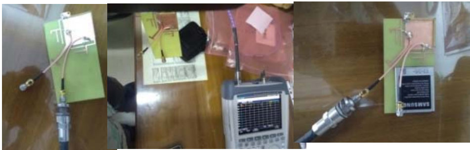
Figure 1. (a) Proposed antenna geometry. (b) Fabricated antenna with and without battery.
