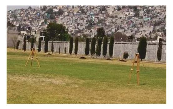
Figure 3. Disposition of radios for a single 50 m straight line, drone (left), GST (right).
