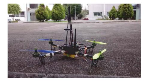
Figure 2. Drone with a 2.4 GHz radio onboard.
