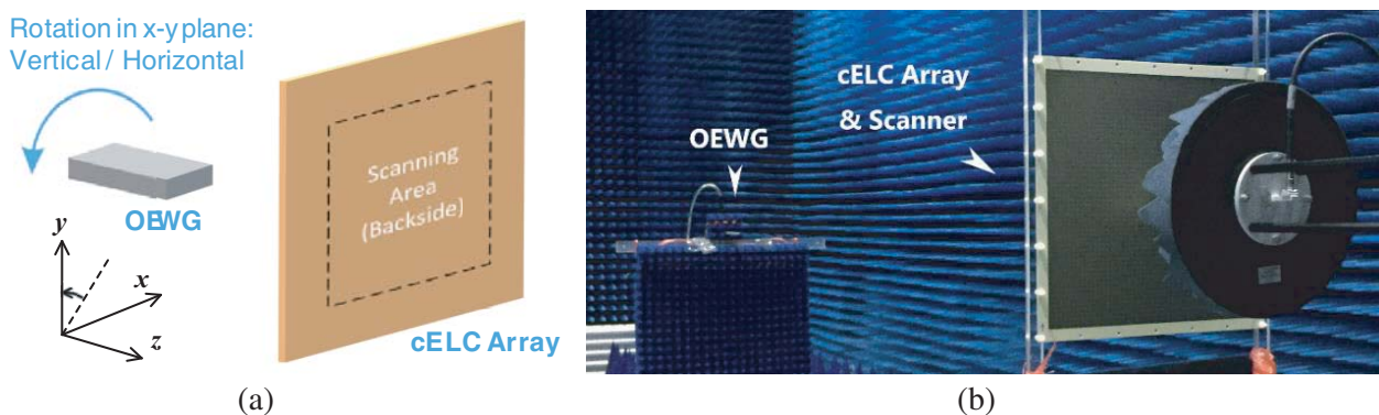
Figure 4. Near-field scanning in a microwave anechoic chamber: (a) schematic diagram; (b) actual scenario.
