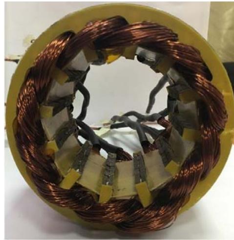
Figure 7. The generator winding frontal parts overhangs.
