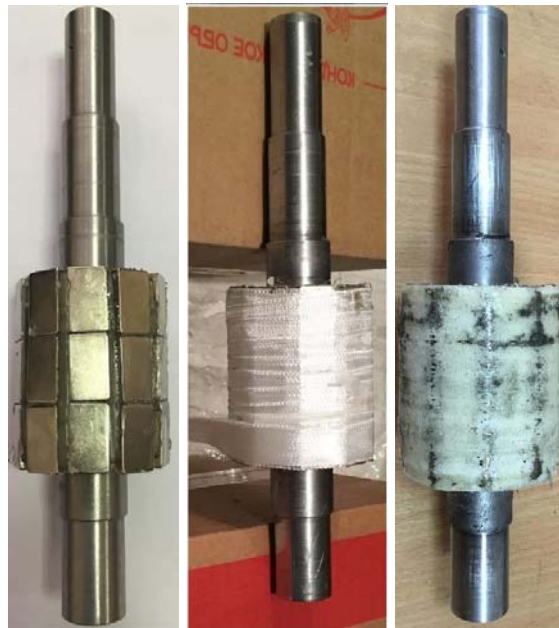
Figure 8. Generator rotor assembly without bandage (left) and with bandage (center and right).
