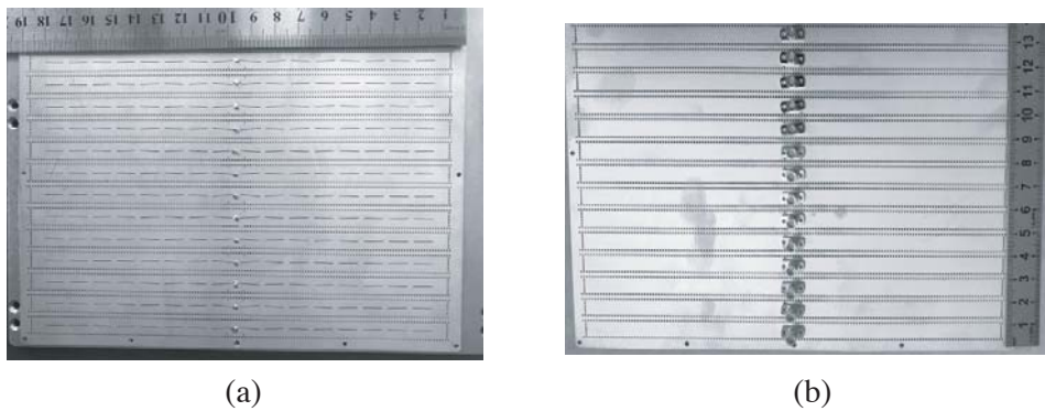
Figure 6. Photograph of the proposed array antenna. (a) Top view. (b) Bottom view.
