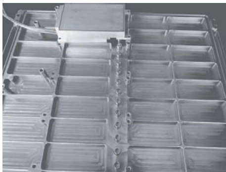
Figure 7. Photograph of the antenna with Tx/Rx module installed.
