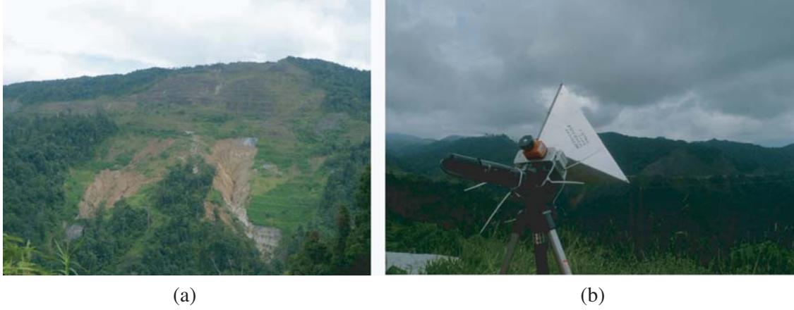
Figure 13. (a) Field measurement test site at Cameron Highland, Malaysia. (b) Trihedral corner reflector as external target.
