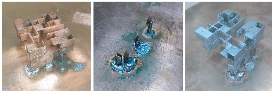
Figure 13. Antenna mounting on 150 \times 150 mm ground plane.
