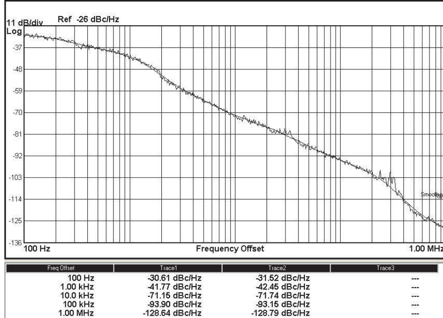
Figure 9. Measured phase noise of the proposed VCO.
