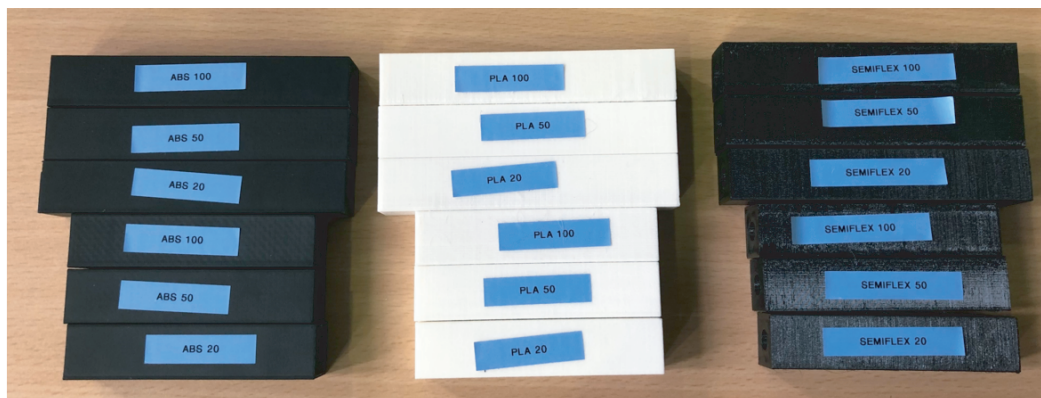
Figure 6. 3D-printed samples different materials and different infill density percentages.
