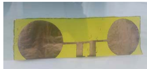
Figure 3. Prototype of the proposed flexible tag antenna.
