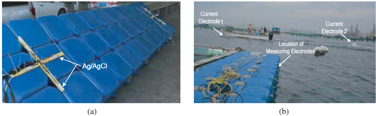
Figure 4. (a) The measuring electrodes are fixed at the bottom of the floating tank and the sea depth of the measuring electrode is 0.2 m; (b) The two current electrodes are towed by a boat at 2.4 m/s.
