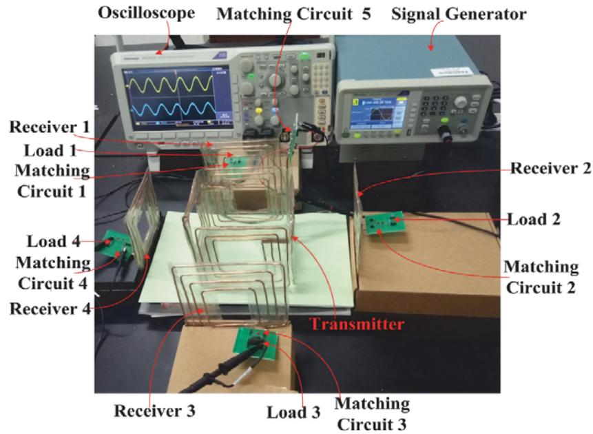
**Figure 10.** The experimental platform of the MRCWPT system.
