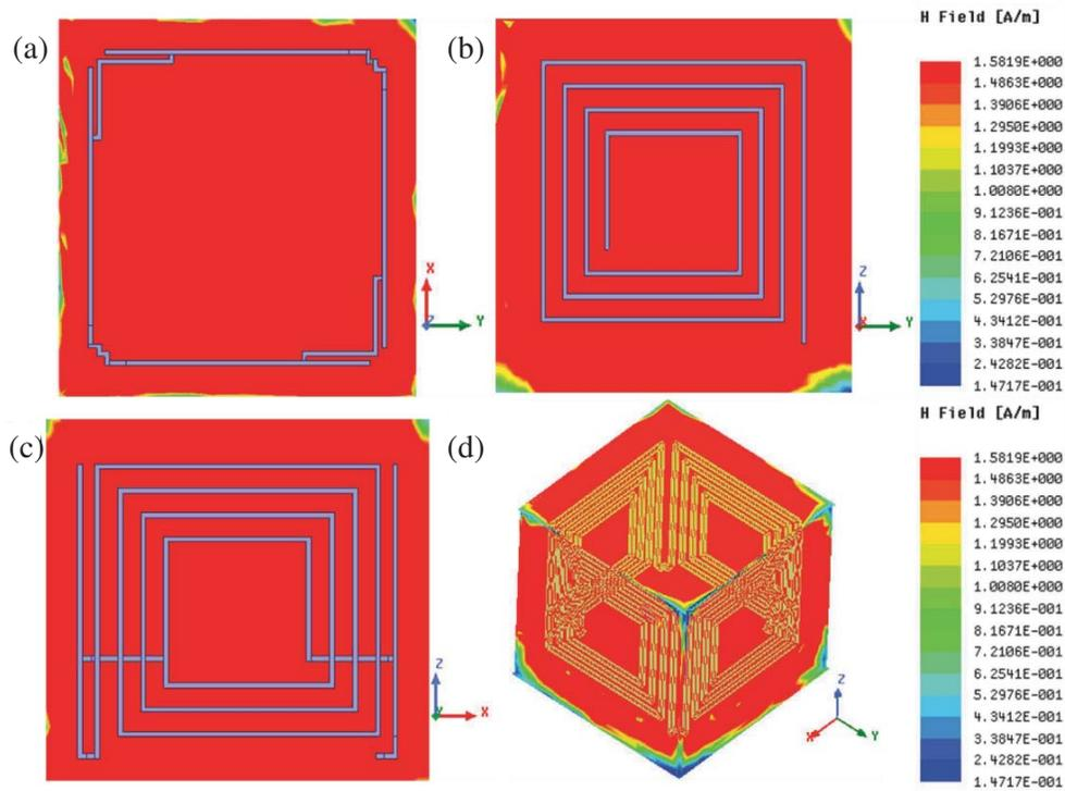
**Figure 6.** The magnetic field distribution of the transmitter.
