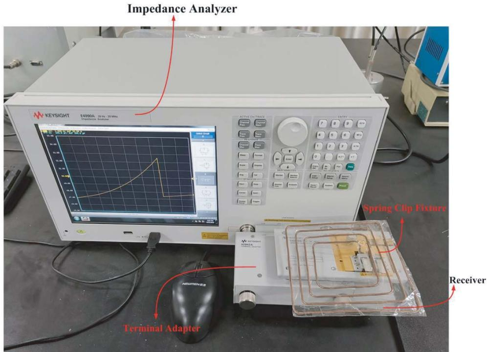
**Figure 11.** The measuring instrument of impedance analyzer (KEYSIGHT E4990A).
