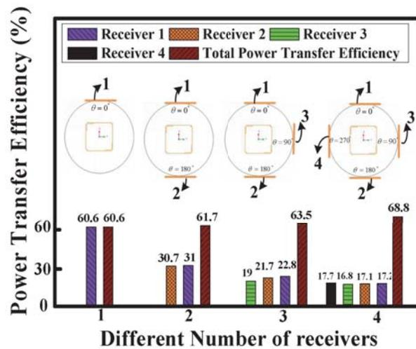
Figure 9. The PTE of the omnidirectional MRCWPT system with different number of receivers.
