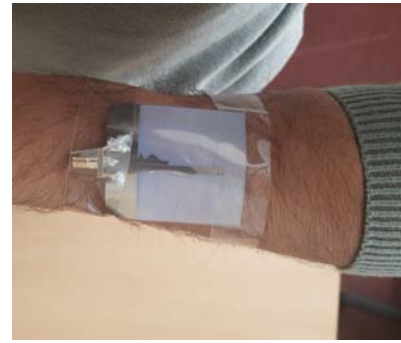
Figure 7. An image of the proposed flexible antenna on top of a subject arm for illustration purposes.
