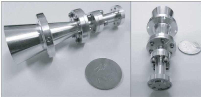
**Figure 4.** Photographs of the fabricated D-band corrugated horn antenna with transition (Iteration 2).
