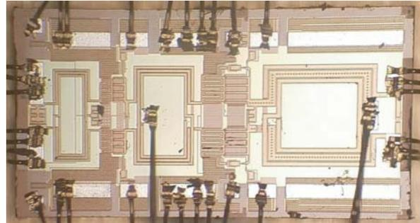
Figure 7. Photograph of the designed CMOS power amplifier.
