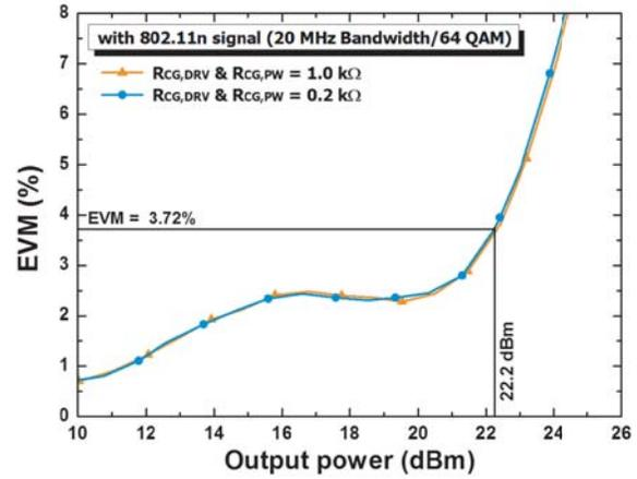
**Figure 11.** Measured results: EVM with 802.11n modulated signal.
