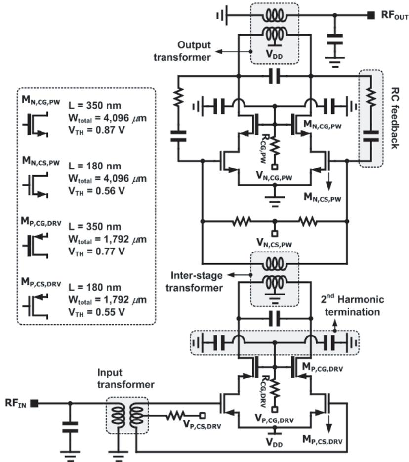
Figure 5. Schematic of designed CMOS power amplifier.
