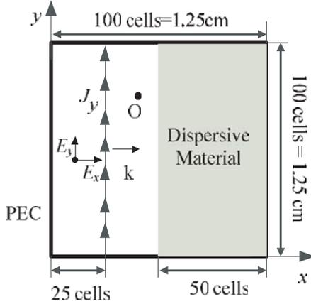
**Figure 1.** Diagram of computational domain for ADE-CN-FDTD.
