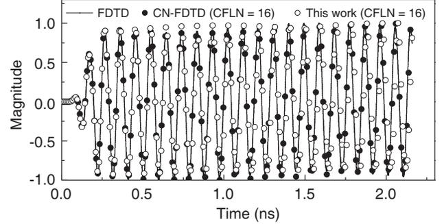
**Figure 2.** The transient fields calculated with conventional ADE-CN-FDTD and the proposed method for Lorentz model.
