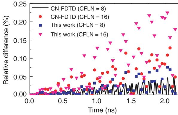
**Figure 3.** The relative difference calculated with conventional ADE-CN-FDTD and the proposed method for Lorentz model.
