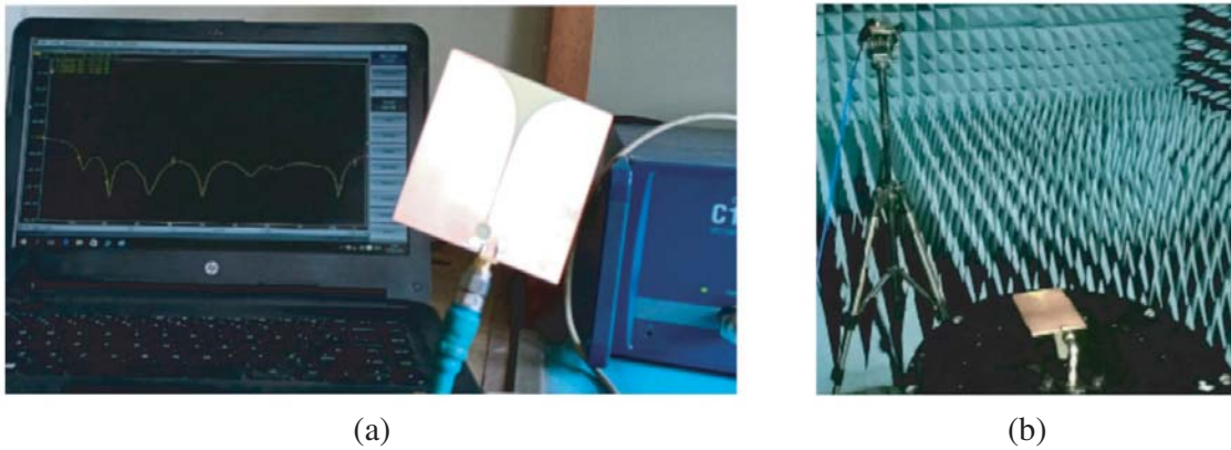
Figure 14. (a) S_{11} measurement and (b) radiation pattern measurement.
