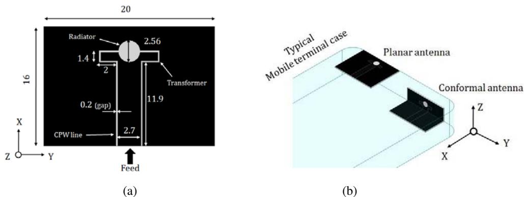
**Figure 1.** (a) Proposed planar antenna (All dimensions are in mm). (b) Comparison of planar and conformal antennas.
