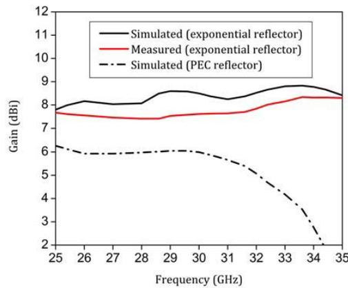
Figure 7. Forward gain of the conformal antenna.
