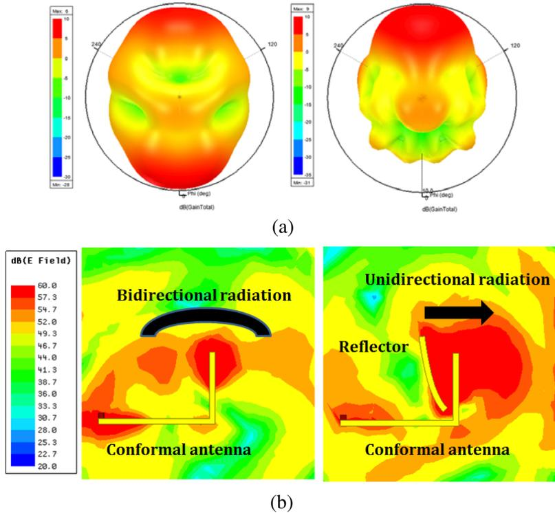
Figure 5. (a) 3D patterns without and with reflector. (b)  $E$ -field plots without and with reflector.
