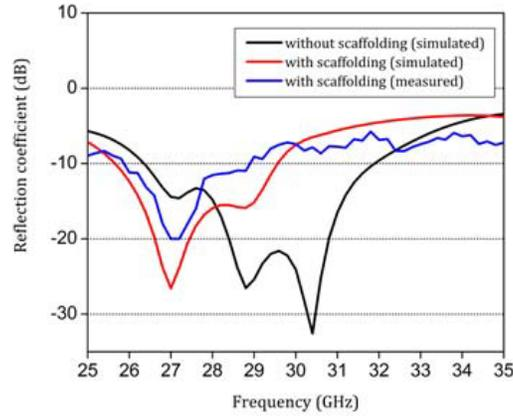
Figure 4.  $|S_{11}|$  of the conformal antenna.
