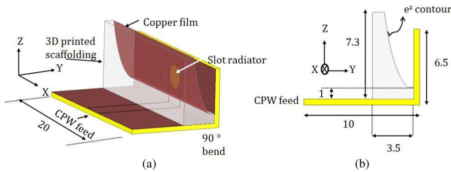
**Figure 2.** Schematic of the proposed conformal antenna. (a) Isometric view. (b) Side view.
