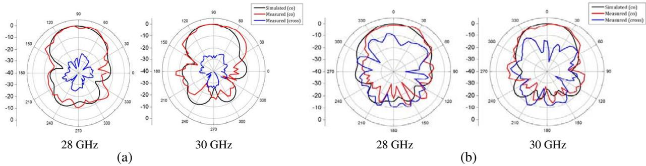
Figure 6. Radiation patterns at 28 and 30 GHz in (a) YZ plane (b) XY plane.
