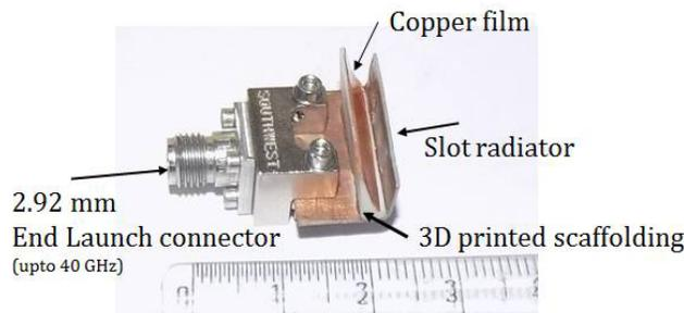
**Figure 3.** Photograph of the fabricated prototype.
