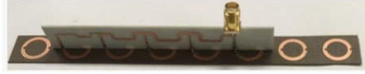
**Figure 5.** Array 1: Generalized Yagi-Uda SRR antenna ( $N_a = 5$ ,  $N_d = 2$ ).
