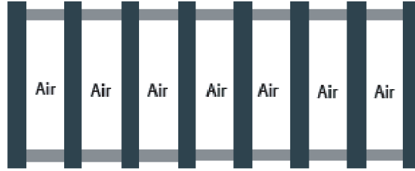
Figure 8. The chosen multilayer structure of type H(LH)^7 with the elementary layers, respectively, Si ( n_H = 3.4 ) and air ( n_L = 1.000256 ).
