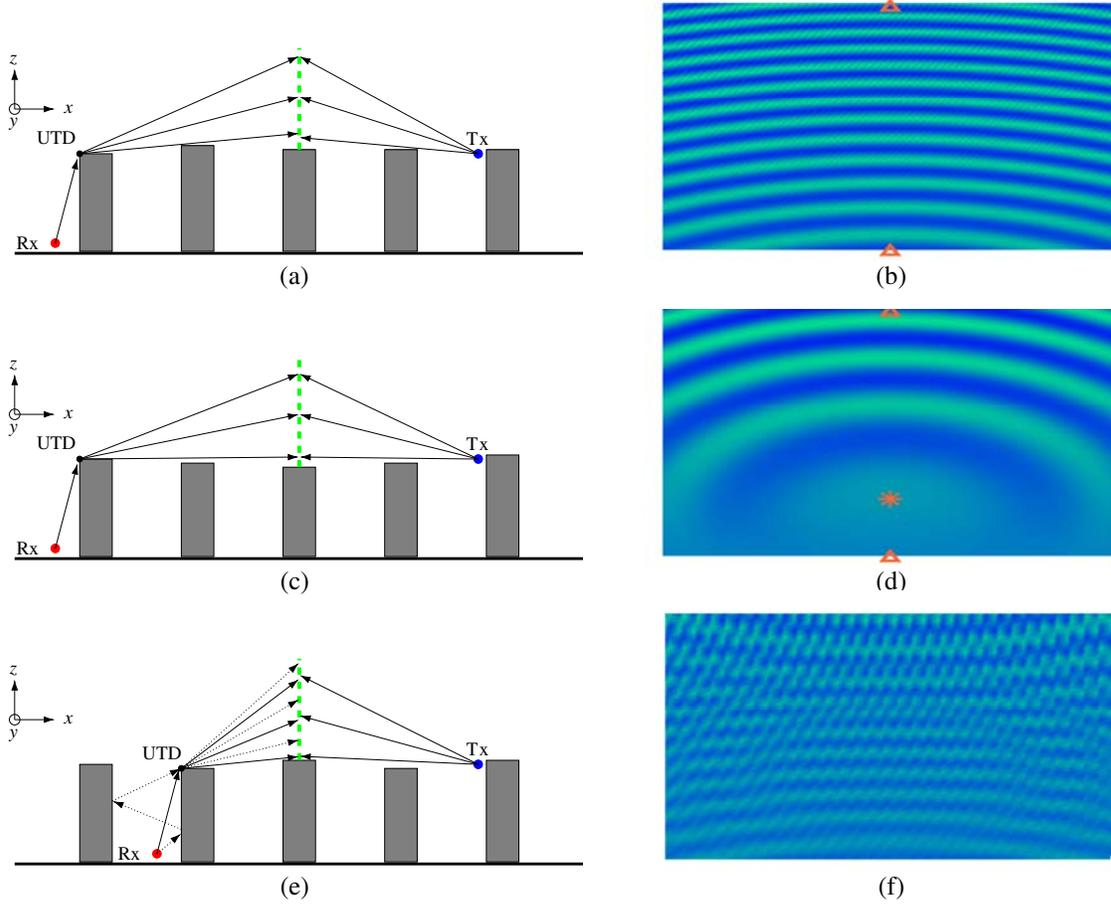
**Figure 5.** Illustration of 3 possible propagation scenarios ((a), (c), (e)) and corresponding  $\text{Re}(\Psi(x))$  (see Eq. (3)) on the interaction surface ((b), (d), (f)). The symbols “\*” and “Δ” denote the locations of the critical points of first and second kind, respectively.
