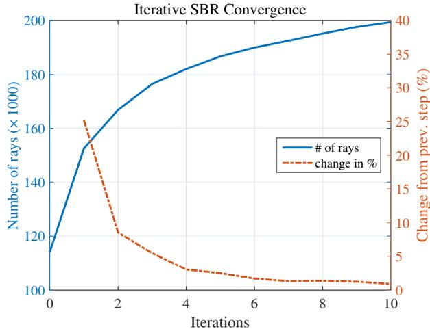
**Figure 6.** Convergence of the iterative SBR algorithm.
