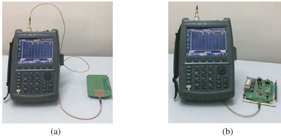
Figure 11. Antenna mounted on router board for return loss measurement. (a) Board bottom view, (b) board front view.
