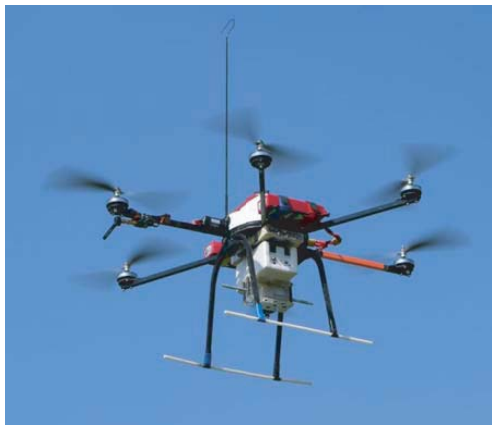
Figure 2. An example of a SUAV with protruded antenna installed.
