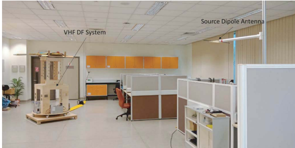
Figure 8. The Direction Finding test setup.
