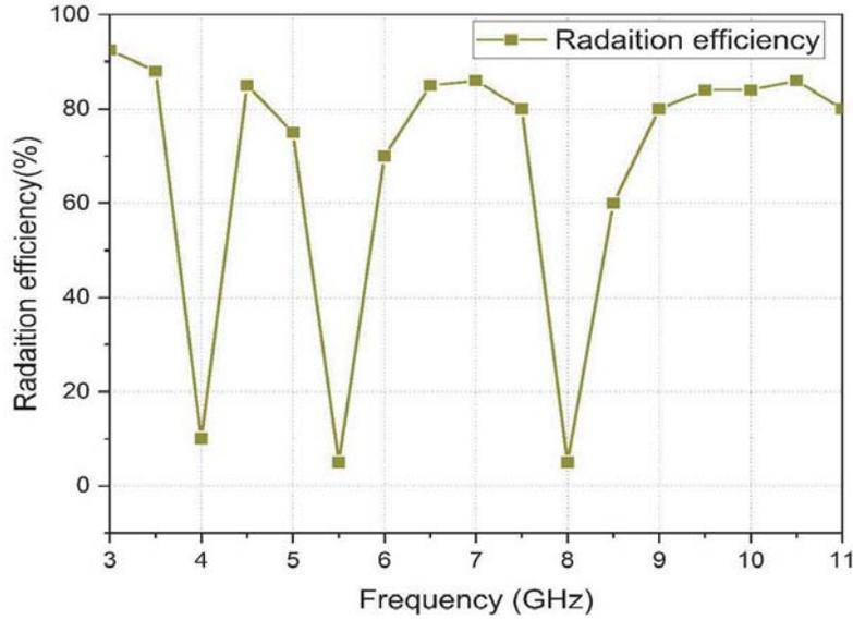
**Figure 16.** Radiation efficiency plot of suggested antenna.
