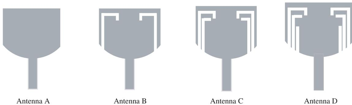
Figure 3. Stepwise expansion of single element UWB antenna (top view).
