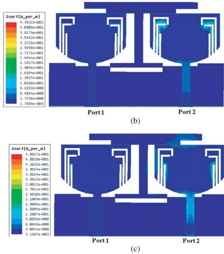
Figure 12. Simulated distribution of surface current (a) 3.7 GHz, (b) 5.5 GHz, (c) 7.5 GHz.
