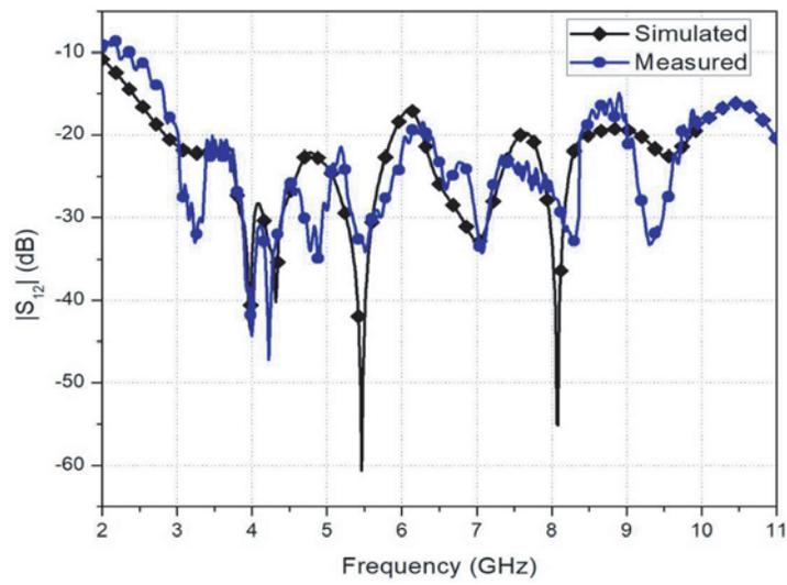
Figure 11. Measured and simulated mutual coupling.
