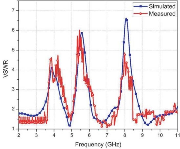
**Figure 5.** Measured and simulated VSWR.
