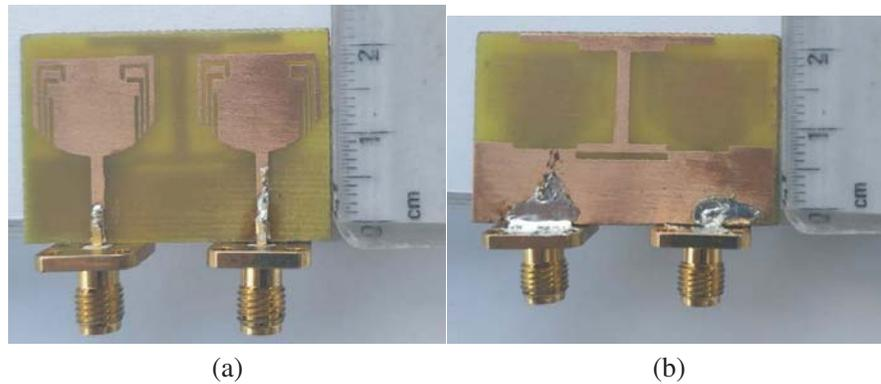
Figure 2. (a) Top view, (b) bottom view of fabricated UWB MIMO antenna.
