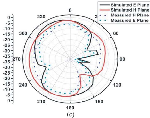
**Figure 13.** Tested and simulated radiation pattern plot of the presented antenna (a) 3 GHz, (b) 5 GHz and (c) 9.5 GHz.
