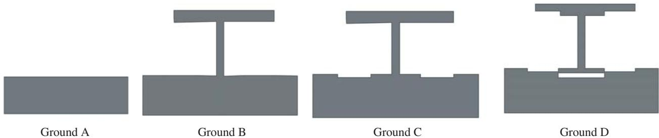
**Figure 9.** Expansion of ground plane of proposed UWB MIMO antenna.
