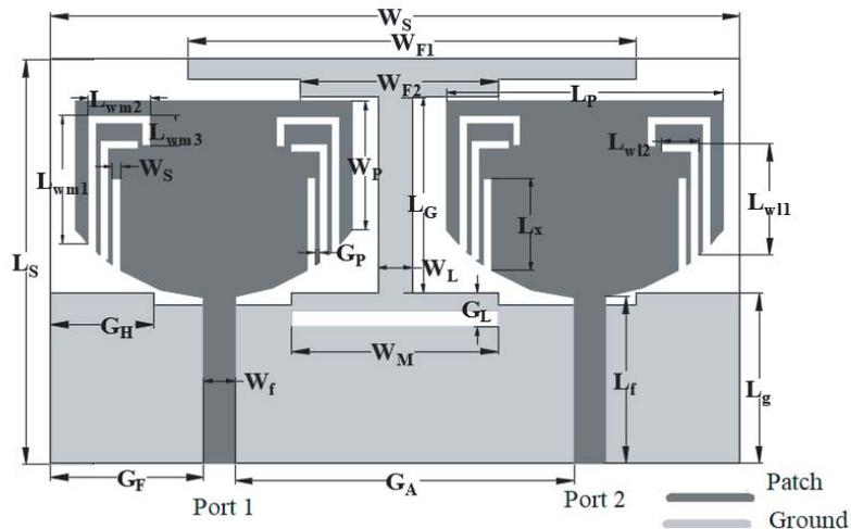
**Figure 1.** Design of suggested antenna.
