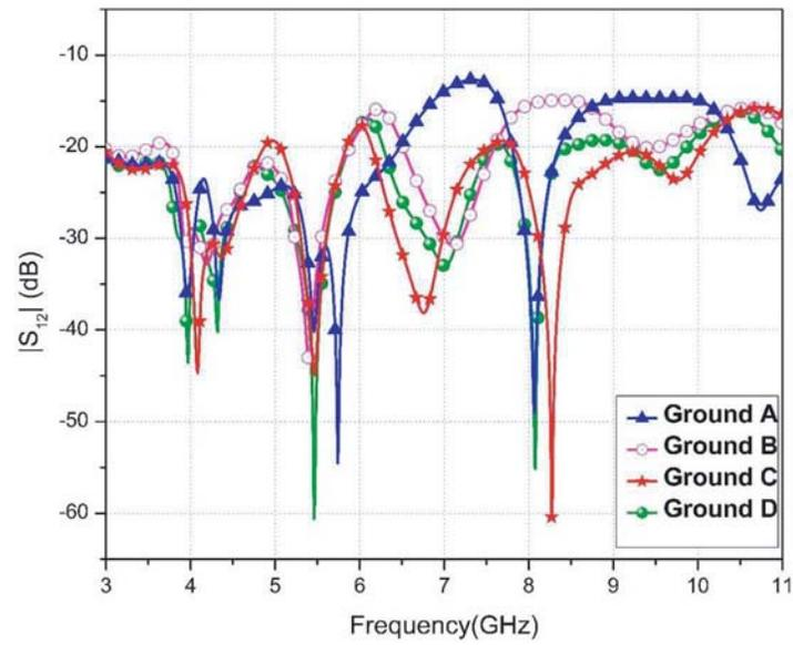
Figure 10. Mutual coupling in dissimilar ground plane.
