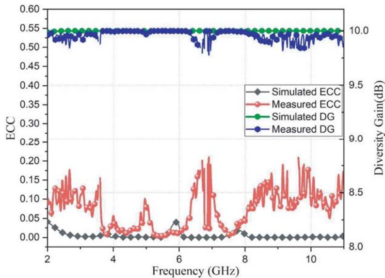
**Figure 14.** Measured and simulated variation of ECC and DG with frequency.
