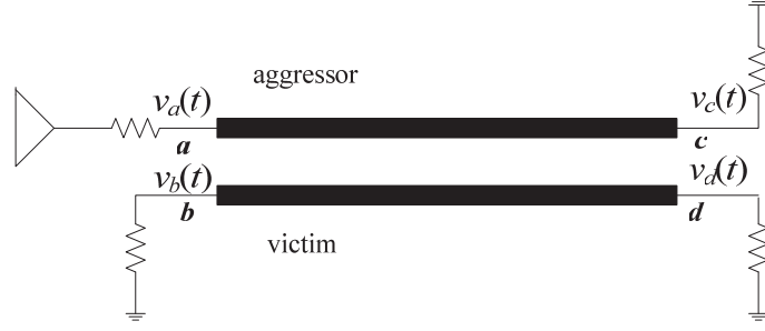
Figure 1. Crosstalk model between the microstrip transmission lines.
