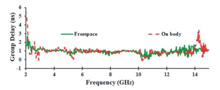
Figure 7. Group delay of the antenna in free space and in close proximity to the body.
