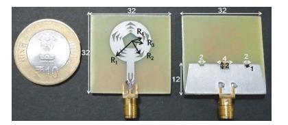
Figure 1. Photograph of the Prototype with dimensional details. (Dimensions are in mm).
