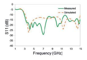
Figure 2. Measured and simulated reflection coefficient of the proposed antenna.
