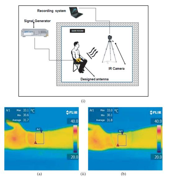
**Figure 9.** Temperature variations for short term EM exposure: (i) Experimental setup and (ii) Sample thermogram: (a) at 0 minute and (b) 20 minutes taken on the right forearm at 6 GHz.
