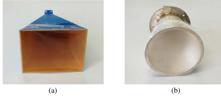
Figure 3. System antennas. (a) The transmitting antenna. (b) The receiving antenna.
