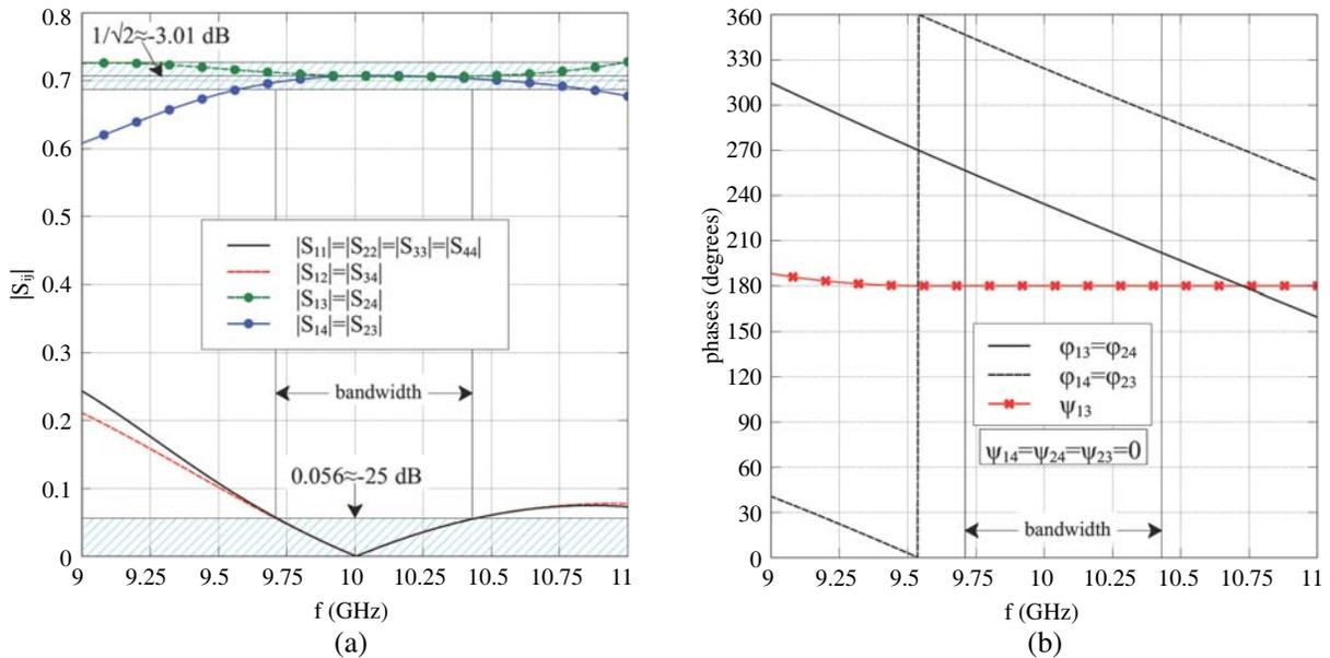
**Figure 2.** Amplitudes  $|S_{ij}|$  (a) and phases  $\varphi_{ij}$  (b) of the scattering coefficients of the 4-port coupler shown in Fig. 1. Elements  $\psi_{ij}$  of the matrix  $\Psi$  are shown in (b).
