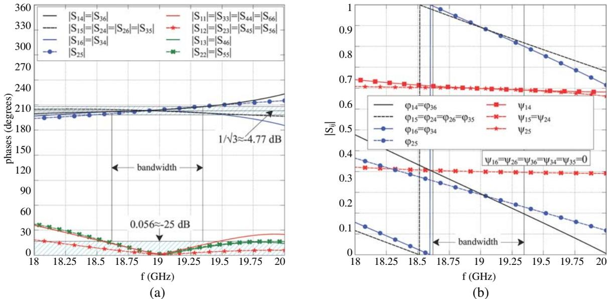
**Figure 4.** Amplitudes  $|S_{ij}|$  (a) and phases  $\varphi_{ij}$  (b) of the scattering coefficients of the 6-port coupler shown in Fig. 4. Elements  $\psi_{ij}$  of the matrix  $\Psi$  are shown in (b).
