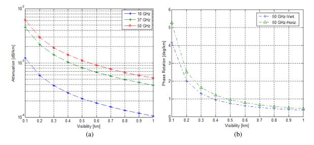
**Figure 3.** (a) Attenuation against visibility using horizontal component (monodisperse medium). (b) Phase rotation against visibility (monodisperse medium).
