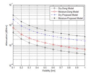
Figure 2. Attenuation against visibility to validate proposed model (polydisperse medium).
