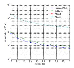
Figure 1. Attenuation against visibility to validate proposed model (monodisperse medium).
