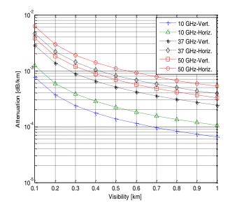
Figure 4. Attenuation against visibility — vertical and horizontal (monodisperse medium).
