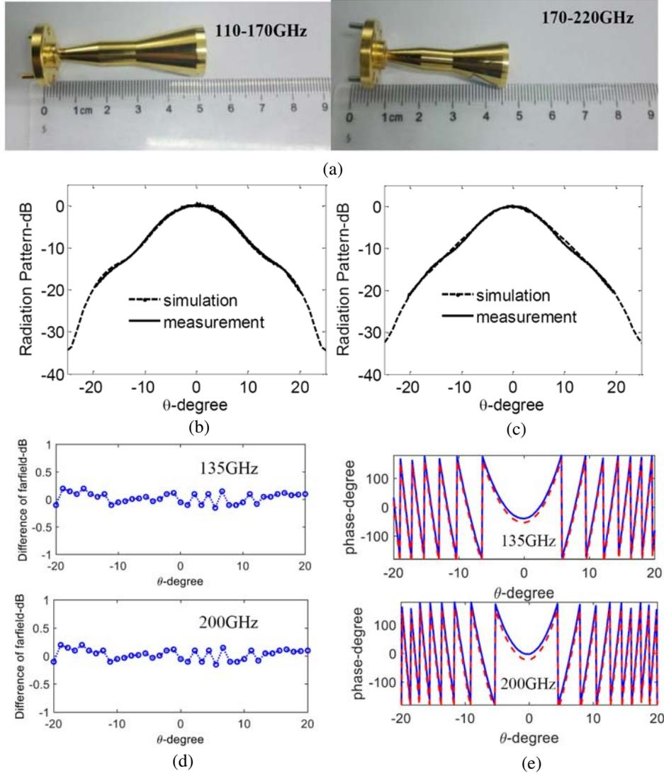
**Figure 10.** Comparison between simulated results and measured results in a non-ideal quiet zone of 2 dB amplitude ripple and  $30^\circ$  phase ripple. (a) Photograph of the horn antennas at 110–170 GHz, and 170–220 GHz. (b) 135 GHz. (c) 200 GHz. (d) Difference between measurement and simulation. (e) The comparison of the measured and simulated phases of the far-field.
