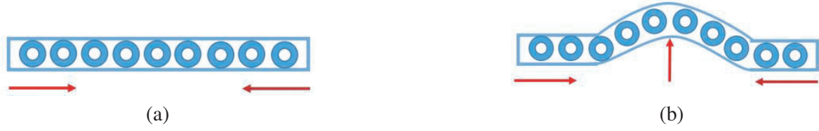
Figure 8. Cross-sectional views showing ply swelling due to interlaminar stress. (a) Interlaminar shear stress a result of moisture uptake, and (b) combined effects of interlaminar shear stress and swelling resulted from moisture absorption.
