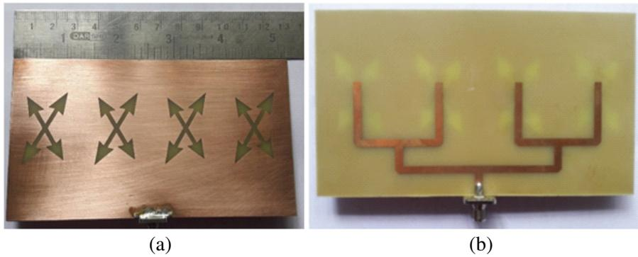
**Figure 7.** Fabricated structure of the proposed modified slot array antenna (a) top view (b) bottom view.
