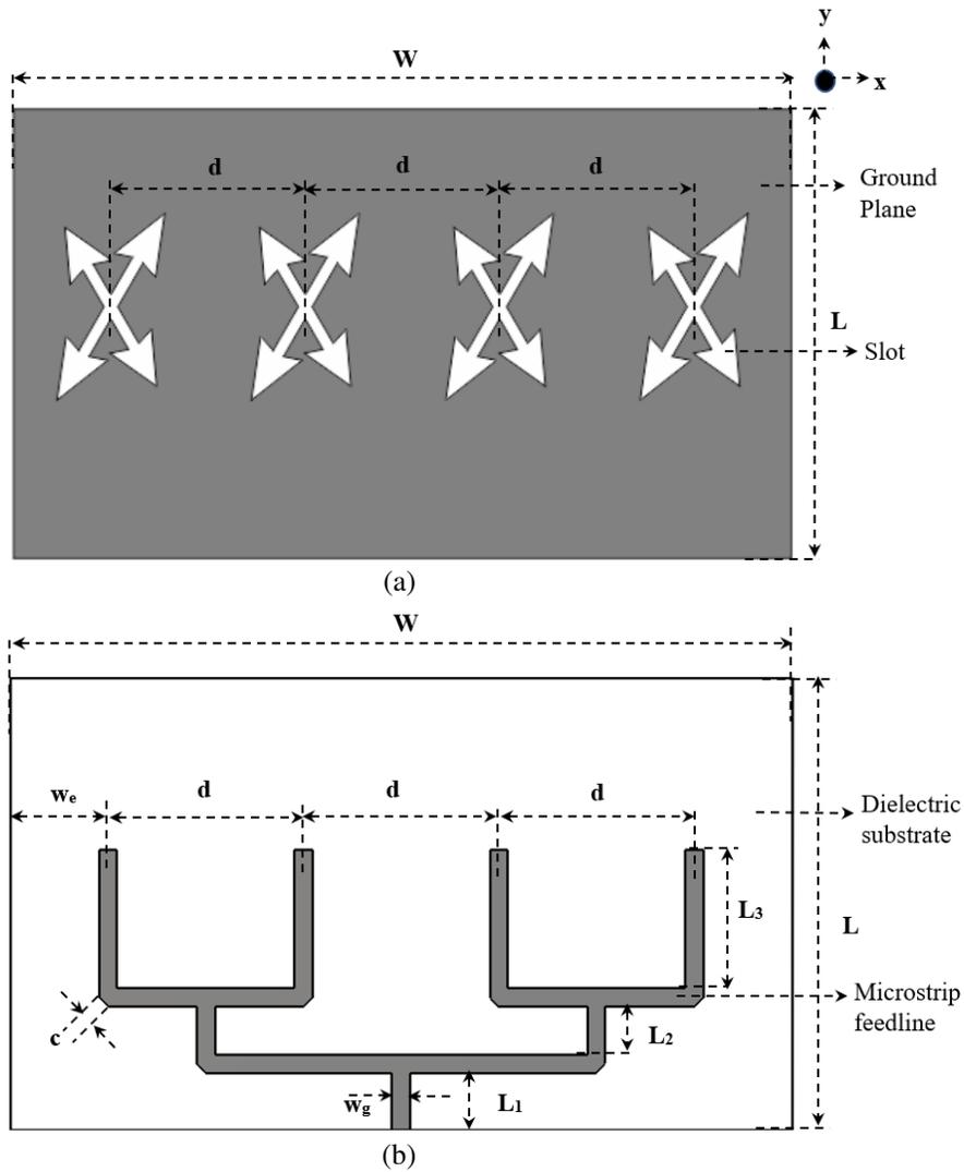
**Figure 1.** Configuration of the proposed arrow headed modified cross slot array geometry (a) top view (b) bottom view.
