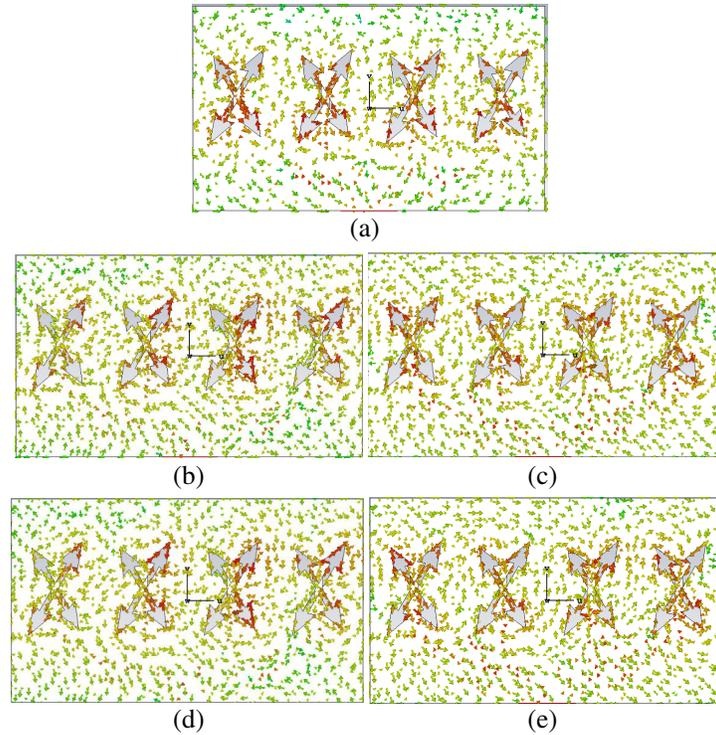
**Figure 4.** Surface current distributions of the proposed modified cross slot array antenna at (a) 1.72 GHz and at 2.45 GHz for (b)  $\theta = 0^\circ$  (c)  $\theta = 90^\circ$  (d)  $\theta = 180^\circ$  (e)  $\theta = 270^\circ$ .
