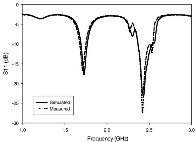
**Figure 5.** Simulated and measured variations of  $S_{11}$  with frequency for the proposed modified slot array antenna.
