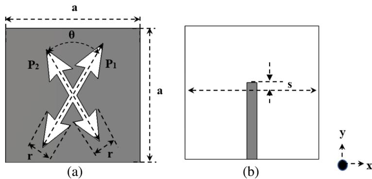
**Figure 2.** Geometry of the single element of the slot array (a) top view (b) bottom view. ( $a = 40$  mm,  $P_1 = 36$  mm,  $P_2 = 31.6$  mm,  $r = 8$  mm,  $\theta = 60^\circ$ ,  $s = 3$  mm).
