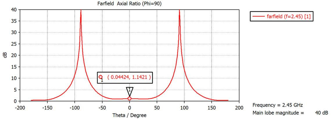
**Figure 3.** Simulated axial ratio (AR) of the proposed slot array antenna at  $f_r = 2.45$  GHz.
