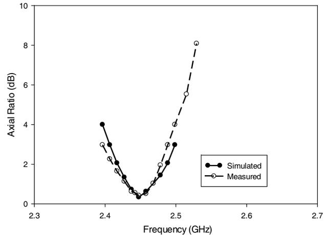
**Figure 6.** Simulated and measured variations of axial ratio with frequency for the upper band of the proposed modified slot array antenna.
