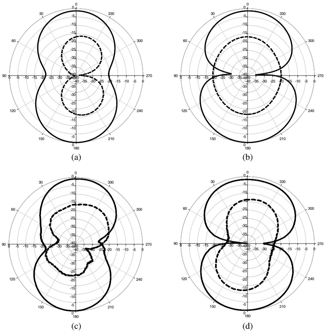
**Figure 8.** Simulated and measured radiation patterns of the proposed modified slot antenna array at 1.72 GHz (a) simulated  $x$ - $z$  plane, (b) simulated  $y$ - $z$  plane, (c) measured  $x$ - $z$  plane, (d) measured  $y$ - $z$  plane. (co-polarised—solid line and cross polarised . . .dashed line).
