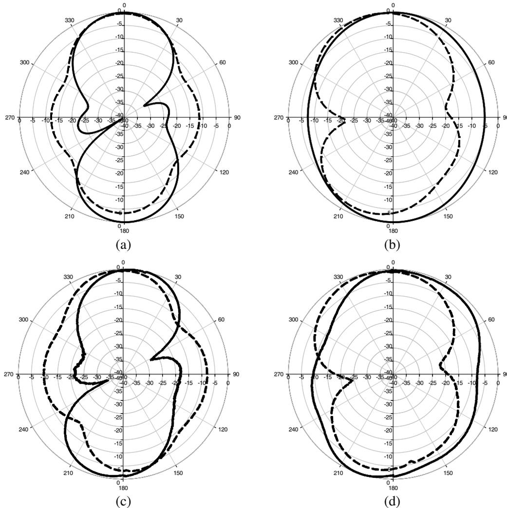
**Figure 9.** Simulated and measured radiation patterns of the proposed modified slot antenna array at 2.45 GHz (a) simulated  $x$ - $z$  plane, (b) simulated  $y$ - $z$  plane, (c) measured  $x$ - $z$  plane, (d) measured  $y$ - $z$  plane. (co-polarised— solid line and cross polarised ...dashed line).
