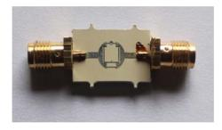
Figure 14. Photograph of fabricated single notch UWB BPF.
