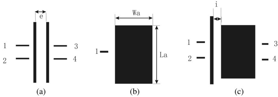
**Figure 2.** (a) Coupled resonators to calculate  $k_{12}$ ; (b) Simulated square patch to obtain  $W_a$  dimension; and (c) patch antenna coupled to resonator to calculate  $k_{23}$ .
