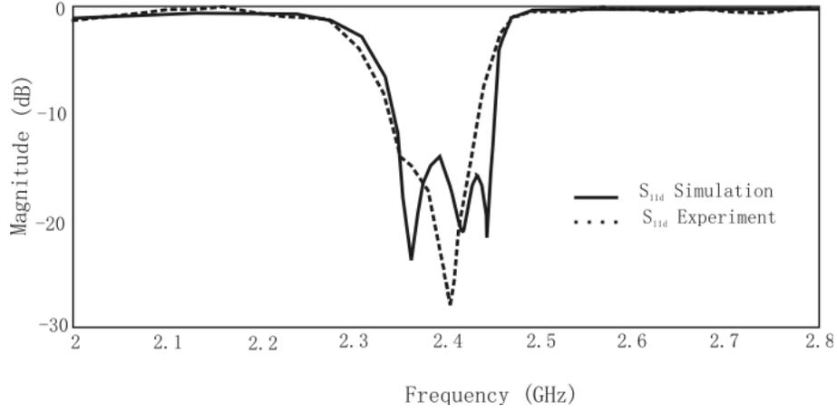
**Figure 4.** Simulated and experimental return losses of filtenna.
