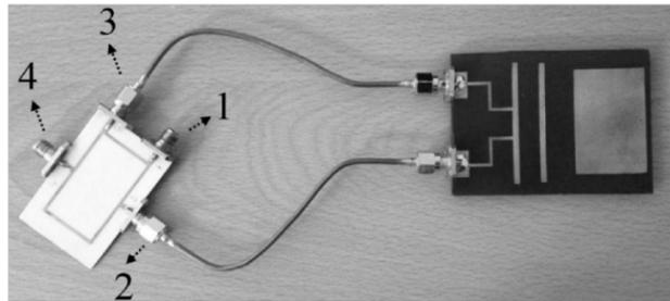
**Figure 3.** Fabricated filtenna connected to hybrid coupler.
