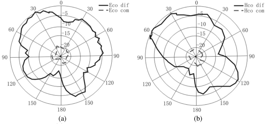
**Figure 5.** Experimental Co-polarized radiation patterns in  $E$  and  $H$  planes for differential and common modes.
