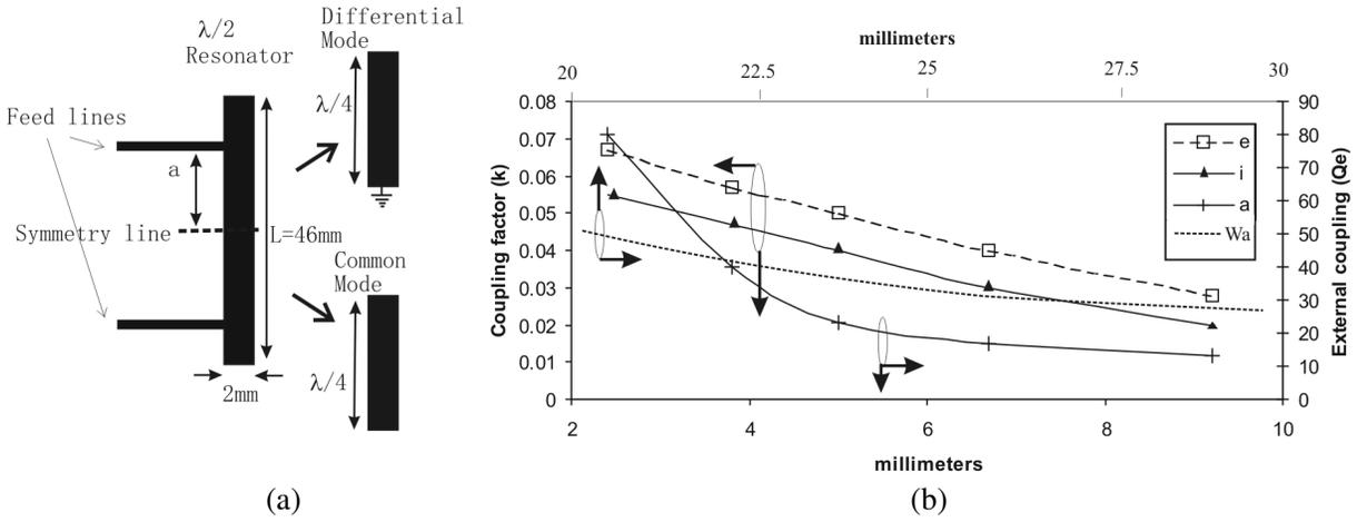
**Figure 1.** (a) Coupled resonator showing differential and common mode operations; (b) simulated mutual coupling, external  $Q$  and radiation  $Q$  values.
