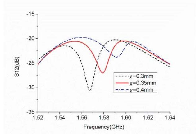
**Figure 6.** The  $S_{12}$  between the antennas when tuning the FDGS slot width.
