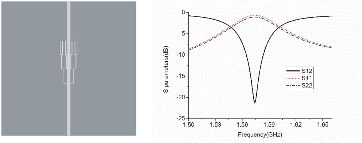
**Figure 3.**  $S$  parameters of designed third iterative FDGS band-gap filter.
