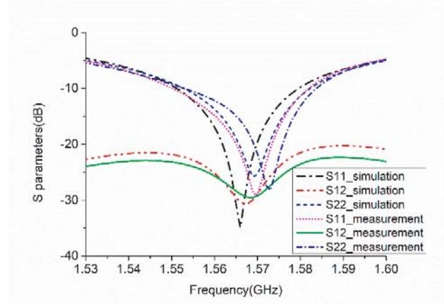
**Figure 11.** The simulated and measured  $S$  parameters with the FDGS.
