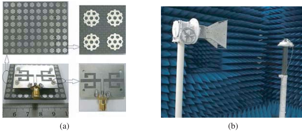
Figure 9. (a) Photograph of the proposed slot antenna and AMC; (b) Experiment environment in the anechoic chamber.
