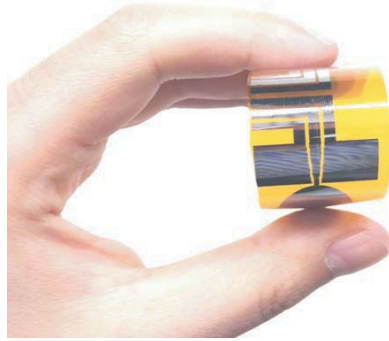
Figure 1. A photo of the proposed Kapton Polyimide based UltraWide Band flexible antenna array.
