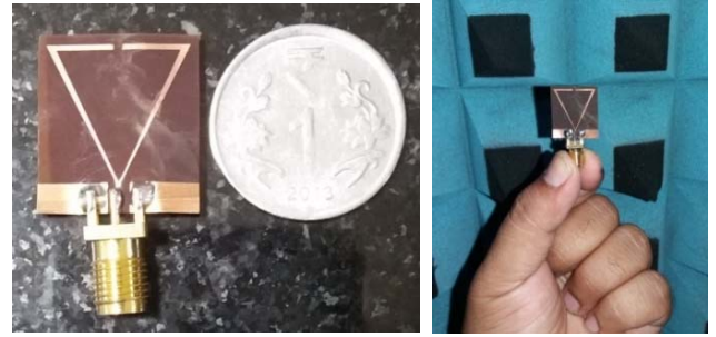
Figure 4. Prototype of fabricated split-triangular patch (STSP) antenna.
