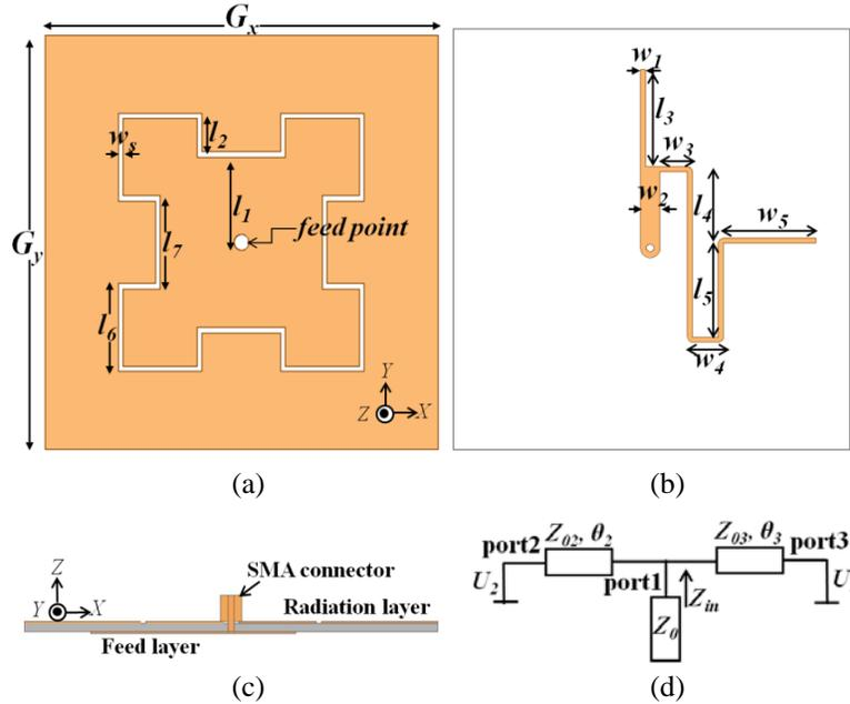
**Figure 1.** Structure of the proposed antenna: (a) radiation layer, (b) feeding network, (c) side view, (d) the equivalent model of the feeding network. ( $G_x = G_y = 80$  mm,  $l_1 = 16.5$  mm,  $l_2 = 8.5$  mm,  $l_3 = 15$  mm,  $l_4 = 11$  mm,  $l_5 = 16$  mm,  $l_6 = 17$  mm,  $l_7 = 18$  mm,  $w_s = 1$  mm,  $w_1 = 0.75$  mm,  $w_2 = 3$  mm,  $w_3 = 5$  mm,  $w_4 = 5.5$  mm,  $w_5 = 15$  mm).
