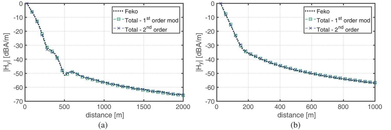
**Figure 6.** (a) and (b) Decay of the magnetic field radiated by an infinite line source of vertical electric Hertzian dipoles over soils: with low negative permittivities at 10 MHz. (a)  $\varepsilon_{rr} = -4$ ;  $\sigma = 0.001$  S/m. (b)  $\varepsilon_{rr} = -2$ ;  $\sigma = 0.001$  S/m.
