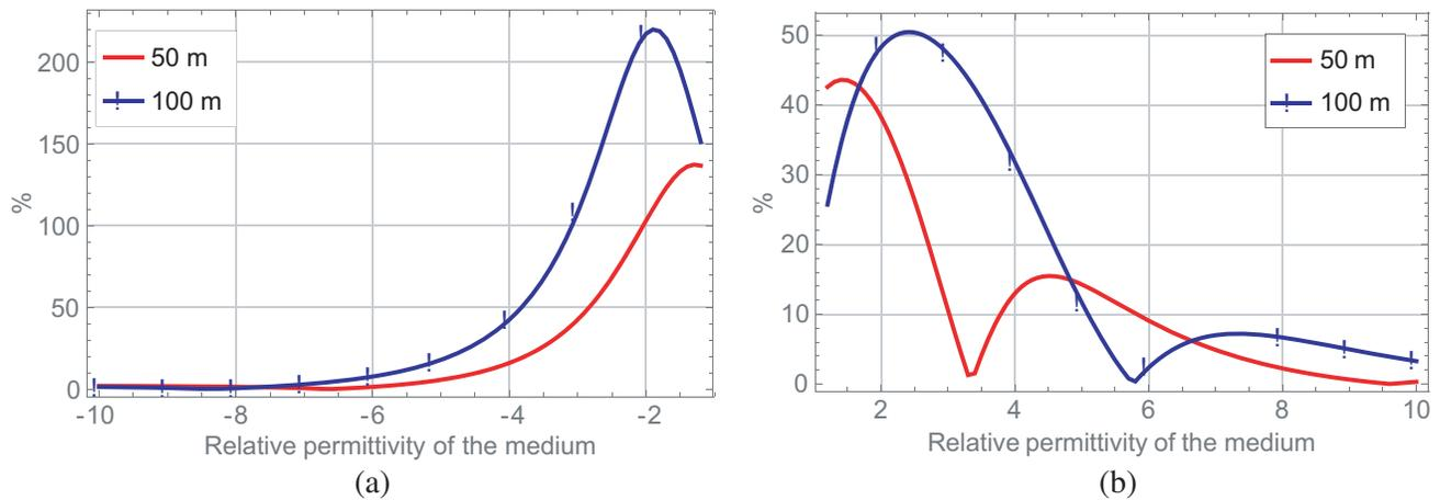
**Figure 7.** Relative error between the magnetic fields obtained with first and second order conditions at 50 m and 100 m (a) with a negative real part of permittivity and (b) with a positive real part of permittivity.
