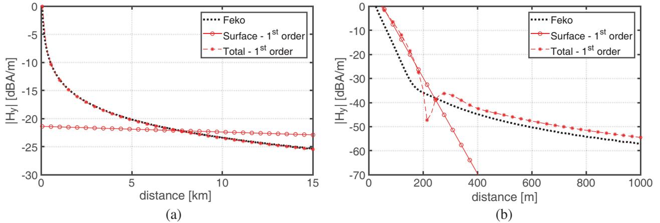
**Figure 4.** Decay of the magnetic field radiated by an infinite line source of Hertzian dipoles over soils (a) with a large positive permittivity and (b) with a low negative permittivity at 10 MHz. (a)  $\epsilon_{rr} = 81$ ;  $\sigma = 5 \text{ S/m}$ . (b)  $\epsilon_{rr} = -2$ ;  $\sigma = 0.001 \text{ S/m}$ .
