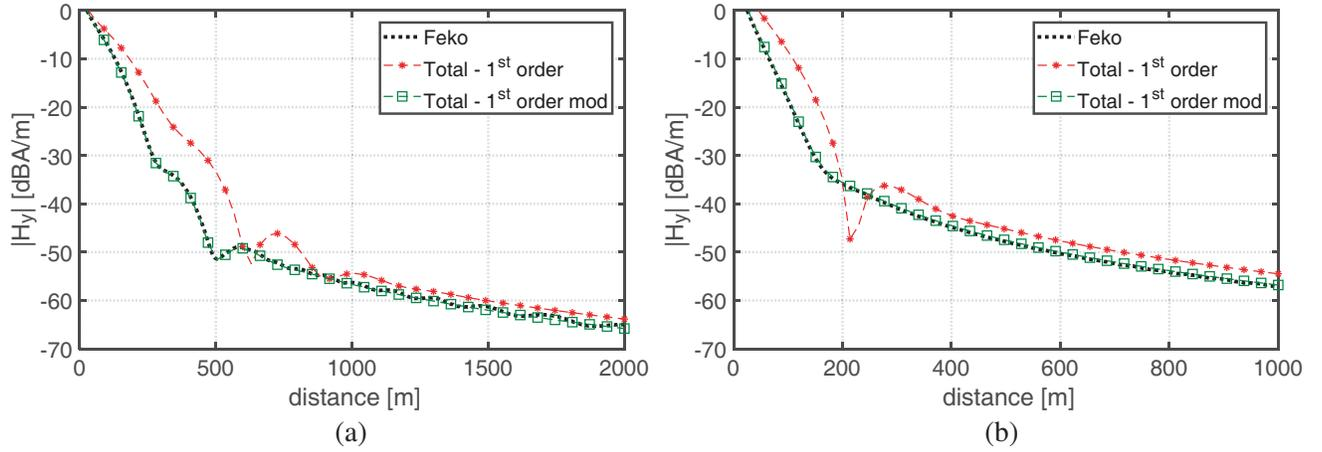
**Figure 5.** (a) and (b) Decay of the magnetic field radiated by an infinite line source of Hertzian dipoles over soils with low negative permittivities at 10 MHz. (a)  $\varepsilon_{rr} = -4$ ;  $\sigma = 0.001$  S/m. (b)  $\varepsilon_{rr} = -2$ ;  $\sigma = 0.001$  S/m.
