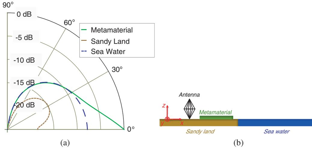
**Figure 2.** (a) shows the distribution of the vertical component of the electric field radiated by a Hertzian dipole located over different grounds, at 10 MHz and at 50 m from the antenna and (b) depicts the side view of the new HFSWR configuration.
