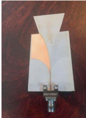
Figure 12. Fabricated modified Vivaldi antenna loaded by ENZ unit cells.
