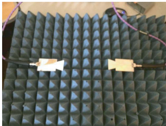
Figure 14. Measurement setup for antenna gain by two-identical antenna method.
