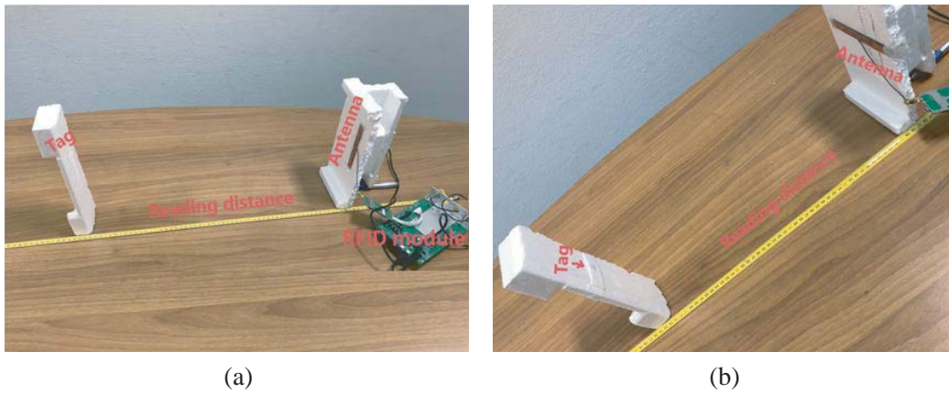
Figure 12. Photography of RFID functional reading distance test of the proposed antenna in (a) vertical, (b) horizontal orientation.
