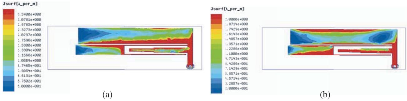
Figure 3. Current distribution. (a) 868 MHz. (b) 2.4 GHz.
