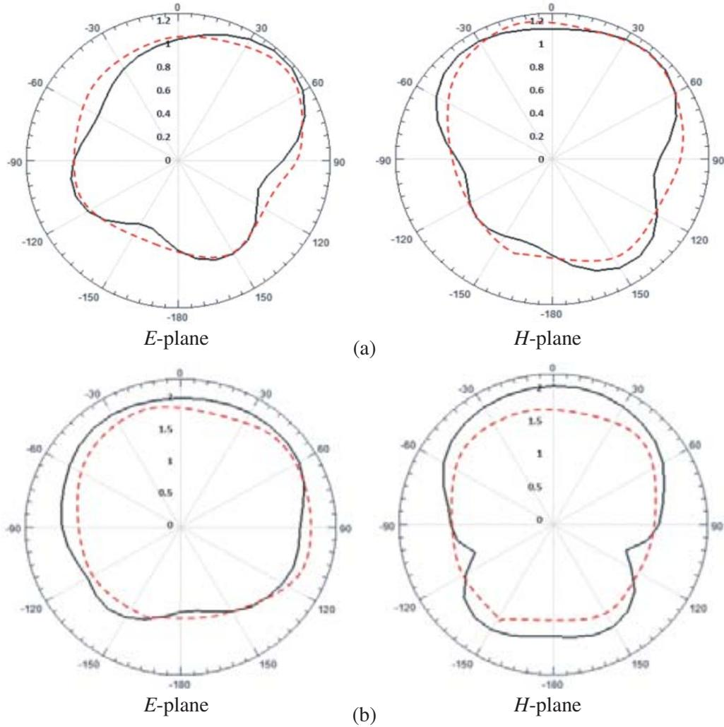
**Figure 7.** Simulated (solid) and measured (dashed) antenna radiation pattern. (a) 868 MHz. (b) 2.4 GHz.
