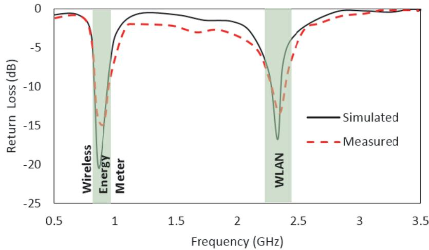
**Figure 2.** Antenna return loss.
