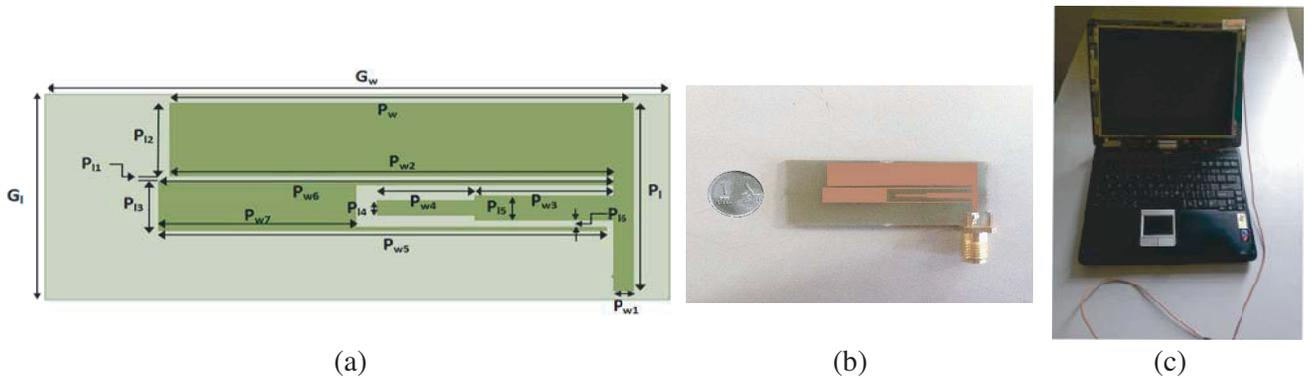
**Figure 1.** Antenna geometry. (a) Top view. (b) Fabricated prototype. (c) Laptop mounting.
