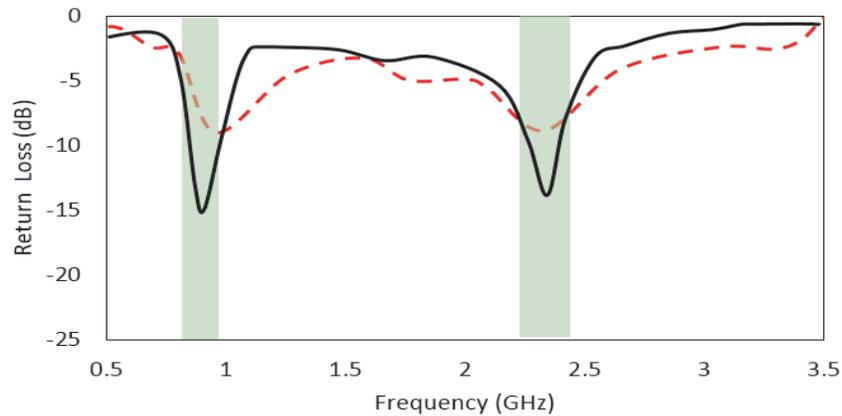
**Figure 6.** Measured return loss when it is free-standing (solid line) and when it is installed in laptop (dashed).
