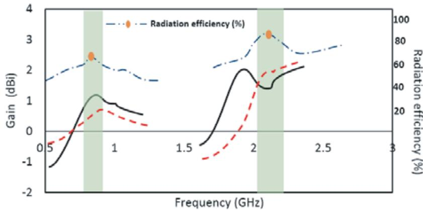
**Figure 5.** Simulated (dashed) and measured (solid) antenna gain.
