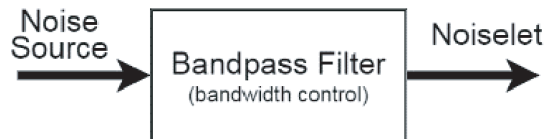
Figure 1. Block diagram of bandpass filtering operation for noiselet generation from noise source (random coefficients) existing over the entire frequency band.
