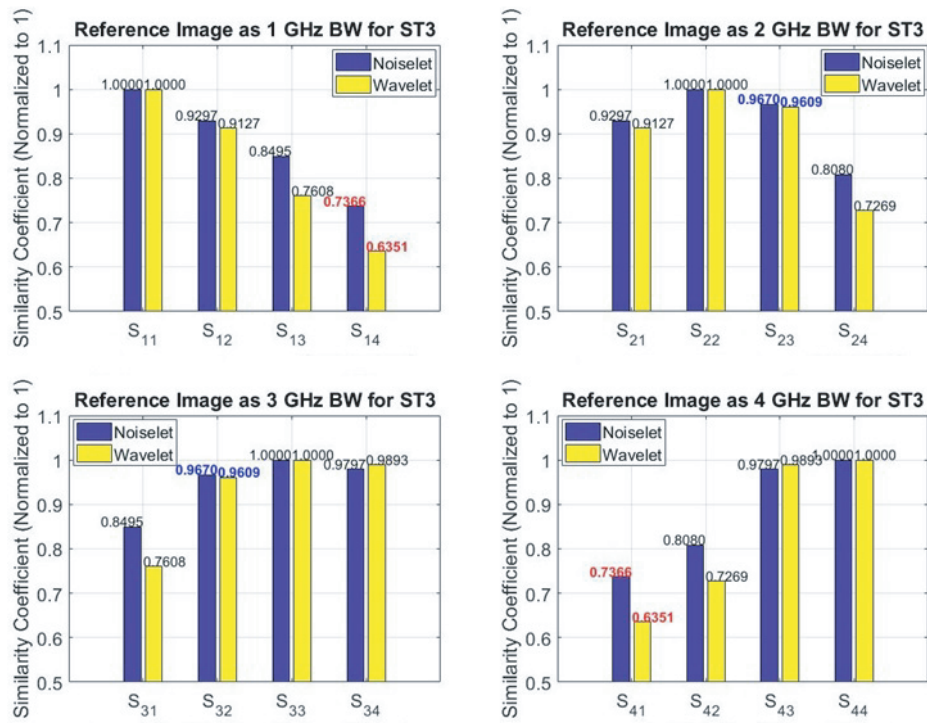
Figure 16. Similarity indices for structure ST3 for different reference images.
