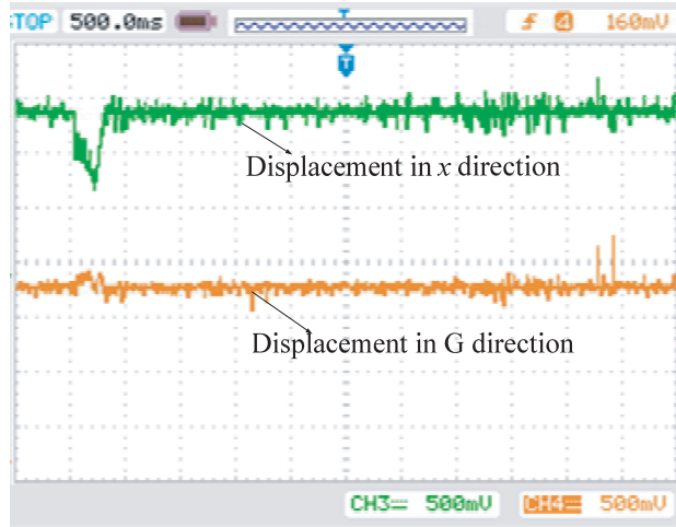
Figure 19. Displacement waves of rotor at the disturbance test.
